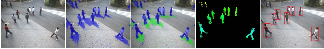
FIGURE 1. Overview of the proposed human detection algorithm based on subtraction stereo. Distance information of foreground regions are obtained from the subtraction stereo through shadow removal (green pixel in the center image). From left to right. Input image, foreground candidate obtained by subtraction stereo, shadow detection, disparity image, detected humans.
